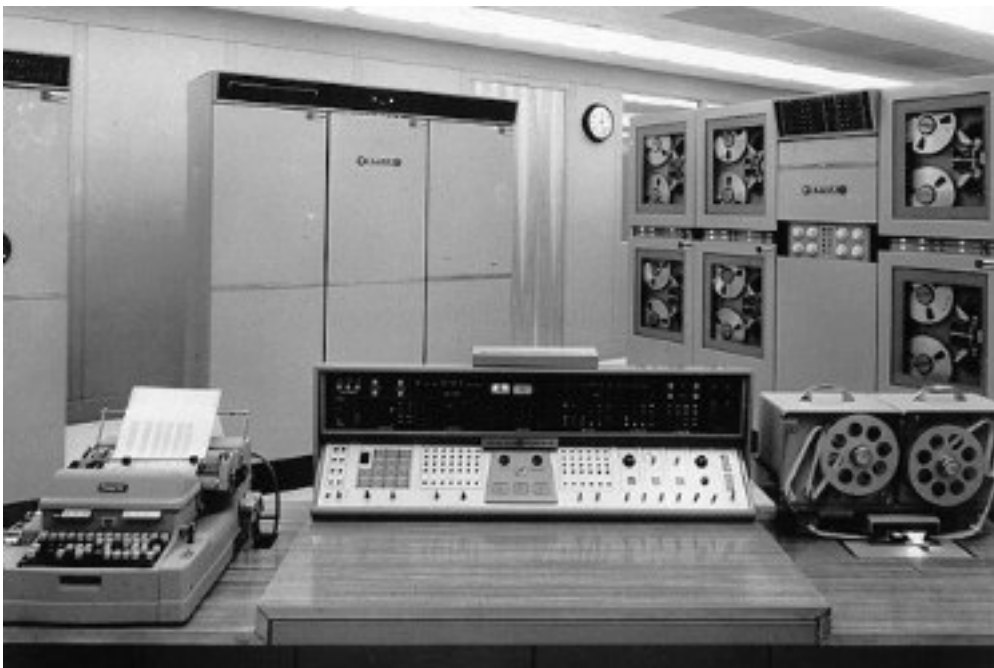
Figure 1.1 Console of General Electric's commercial ERMA
