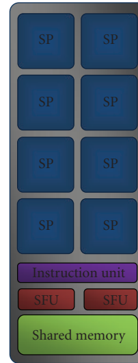
FIGURE 2: Streaming multiprocessors in detail.
