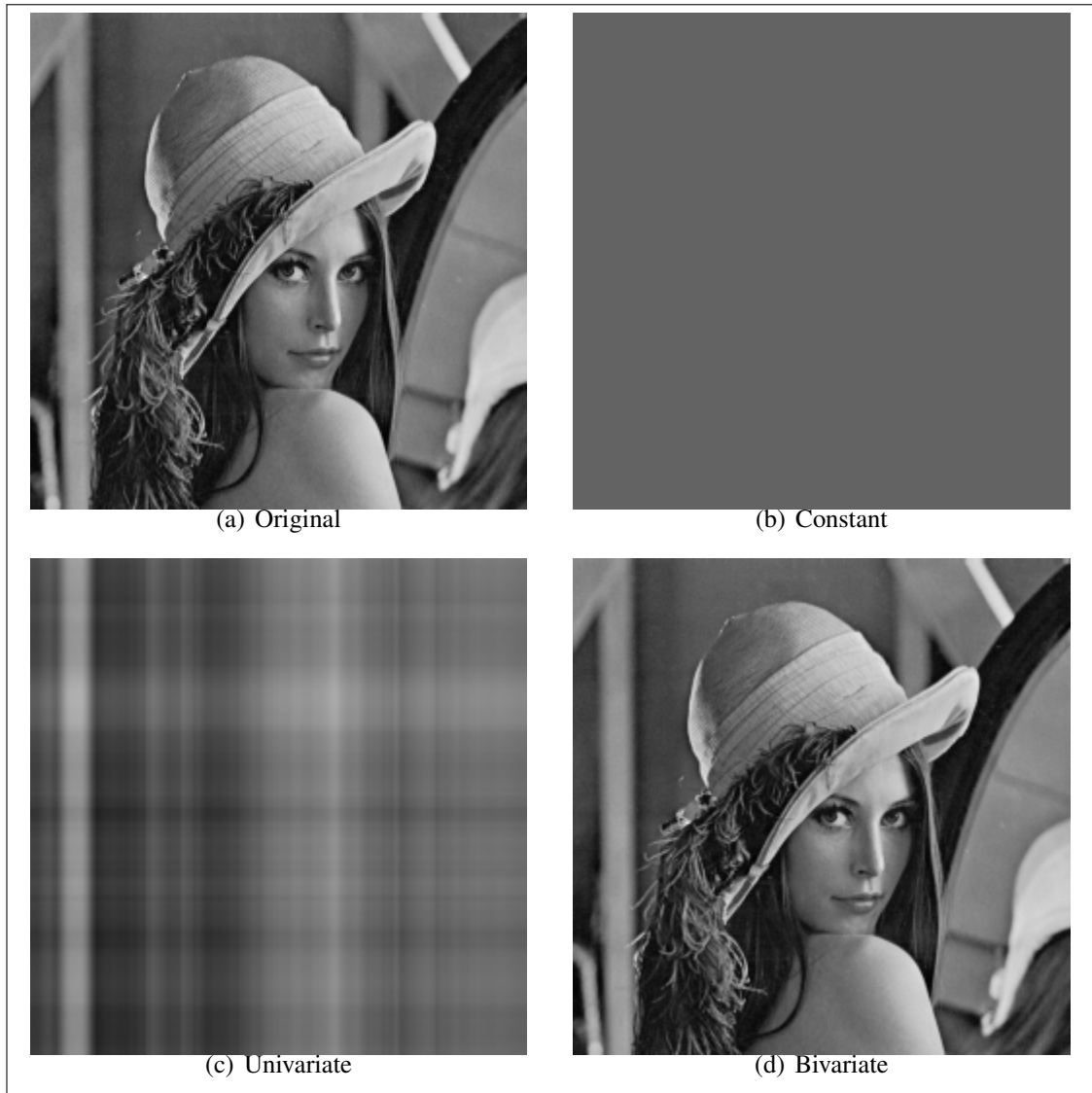
Figure 2.3: Interpolated images by using the terms up to (b) constant term, (c) univariate terms and (d) bivariate terms.
