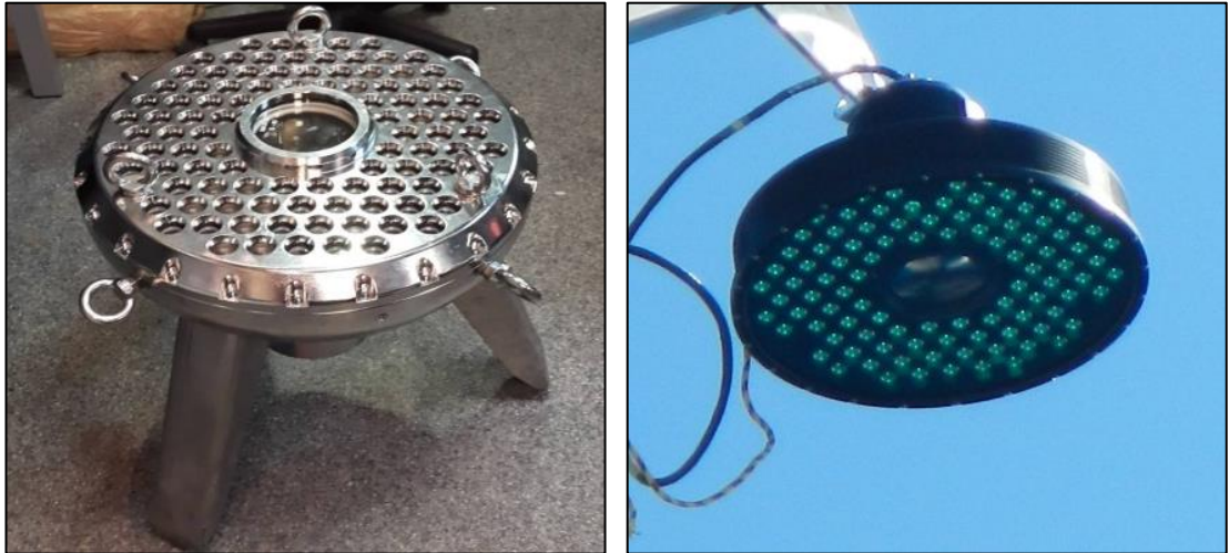
Figure 5.1: The underwater optical communication unit (left) and the free space optical communication unit (right) of the two-way optical communication system.
