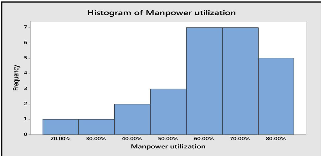
Figure 4.2 shows that twenty out of twenty six observations for OEE calculation for all machines are equal 50 percent or less and all observations are less than 70 percent. Moreover, figure 4.3 shows the uncertainty of manpower utilization calculations. Hence, Machine Interference Problem (MIP) had been discussed in section 4.3 to improve the OEE and manpower utilization to increase productivity and reduce production lead time.
