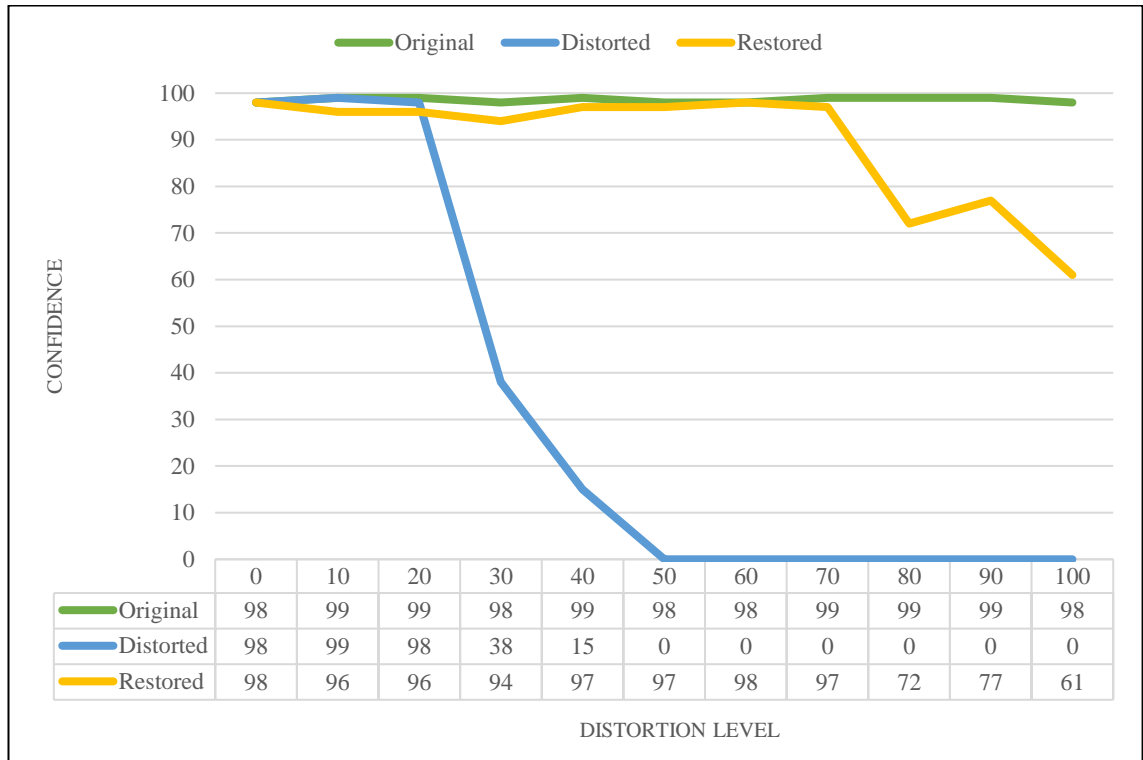
Figure 4.15: Noise restoration performance for MobileNet
