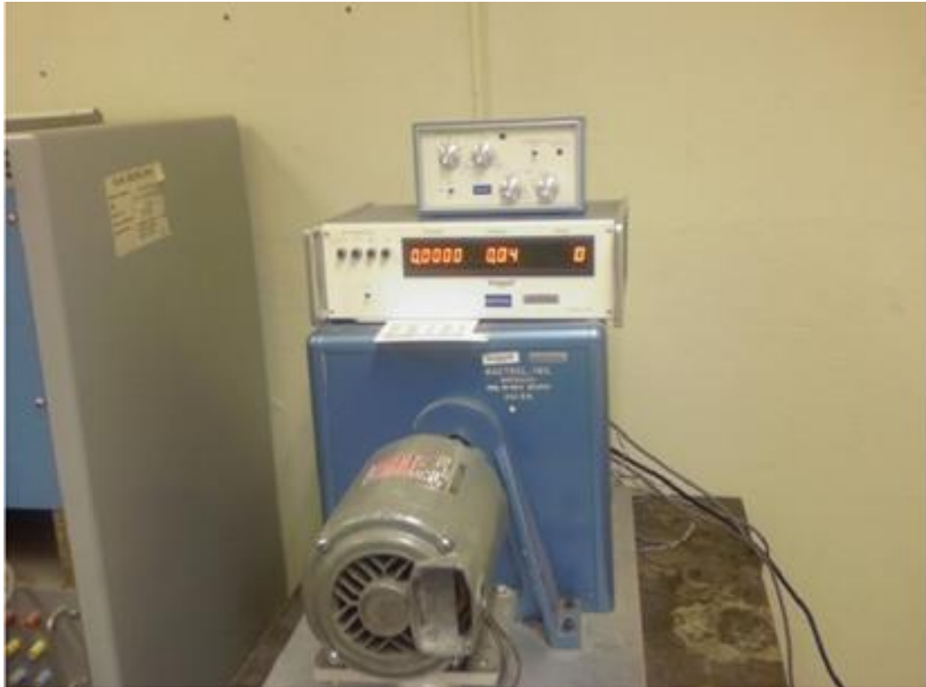
Figure 5.1: Test setup for induction motor with a single broken rotor bar
