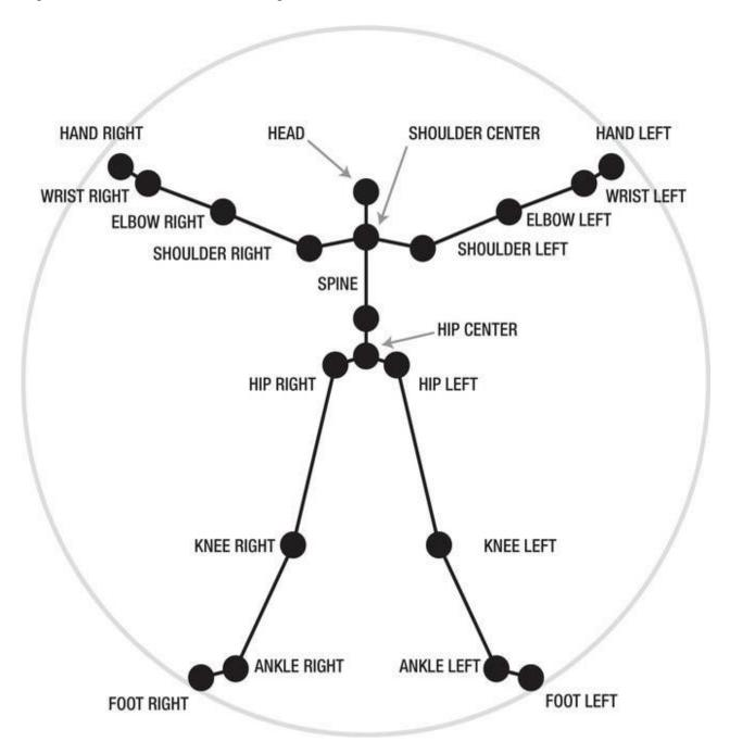
Figure 3.3 : Kinect Skeleton Tracking Joint Positions
