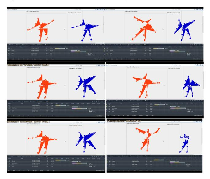
As seen at Figure 6.3 because of the network latency and the data losses the shape of the skeletons deformed.
