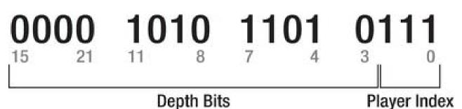
This means for a 640\*480 resolution frame kinect produces 16\*640\*480 bits. Also programmers can determine the player with mask 0000 0111.
