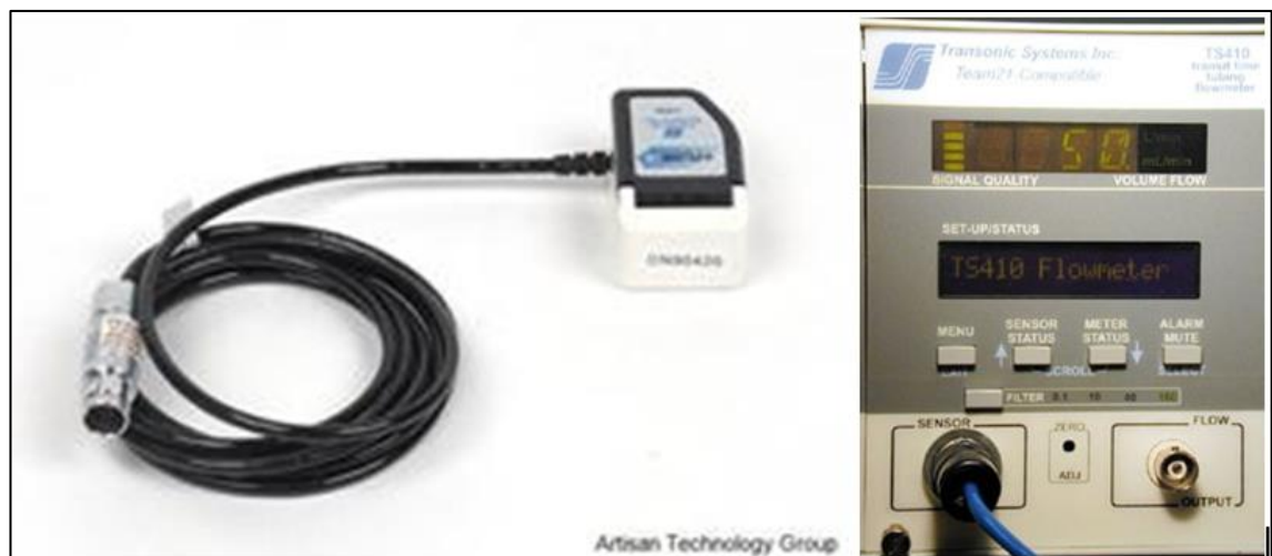
Figure 2.13: Transonic pipe clamp sensor and measurement unit
