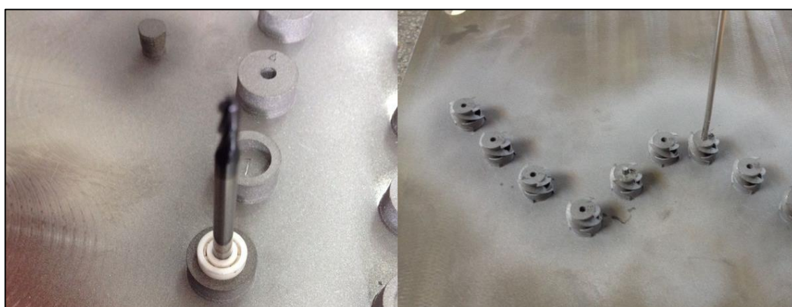
Figure 2.25: Trial particals for determining fitting tolerances
