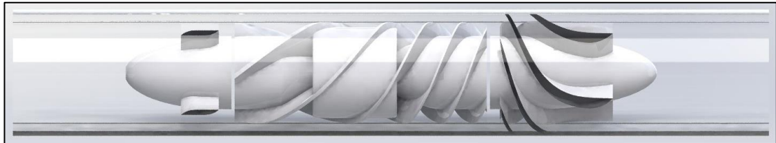
Figure 2.8: Side view of the FP1 inside initial circular shroud
