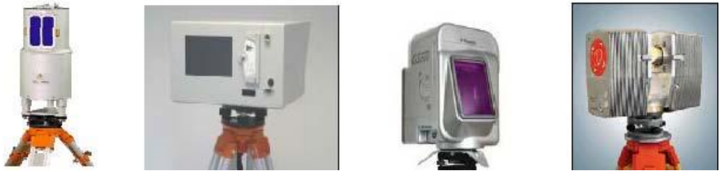
A ) Riegl LMS-Z210i B ) Optech -ILRIS 3D C ) Trimble-(Mensi) GS200 D) IQSun 880
