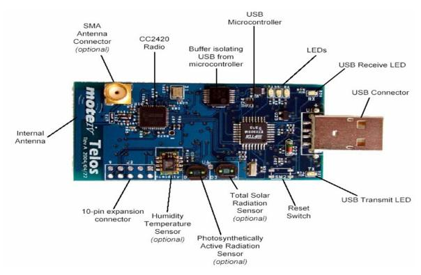
Figure 2.2 : TMote-Sky node used in channel modeling at smart grid environments
