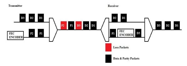
Figure 4.2 : Static FEC mechanism
