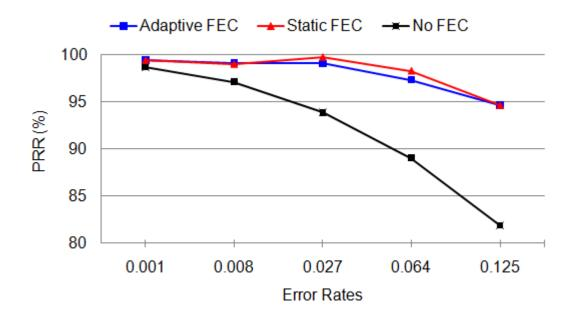
Figure 4.7 : PRR vs. error rates in underground transformer vault
