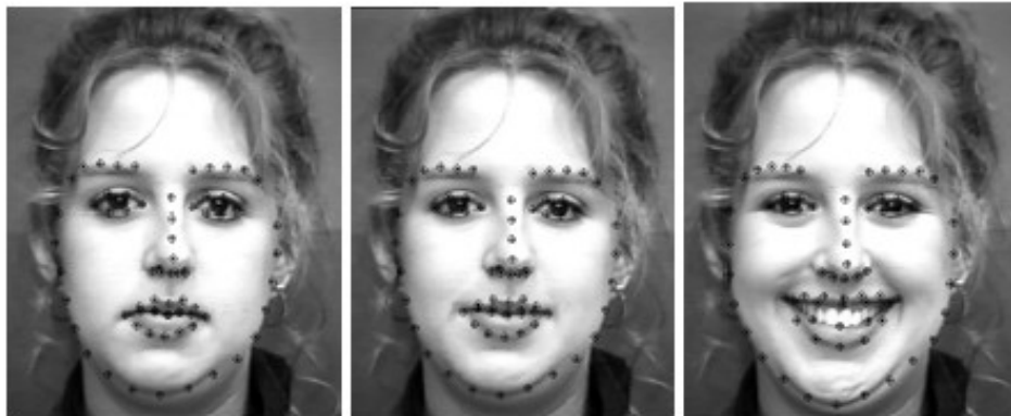
Figure 3.1 : AAM based tracking of landmark coordinates in CK+ database 1st, 5th, and 33rd frames respectively from left to right
