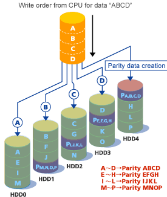
Figure 1-6 RAID 5 structure – distributed data guarding
