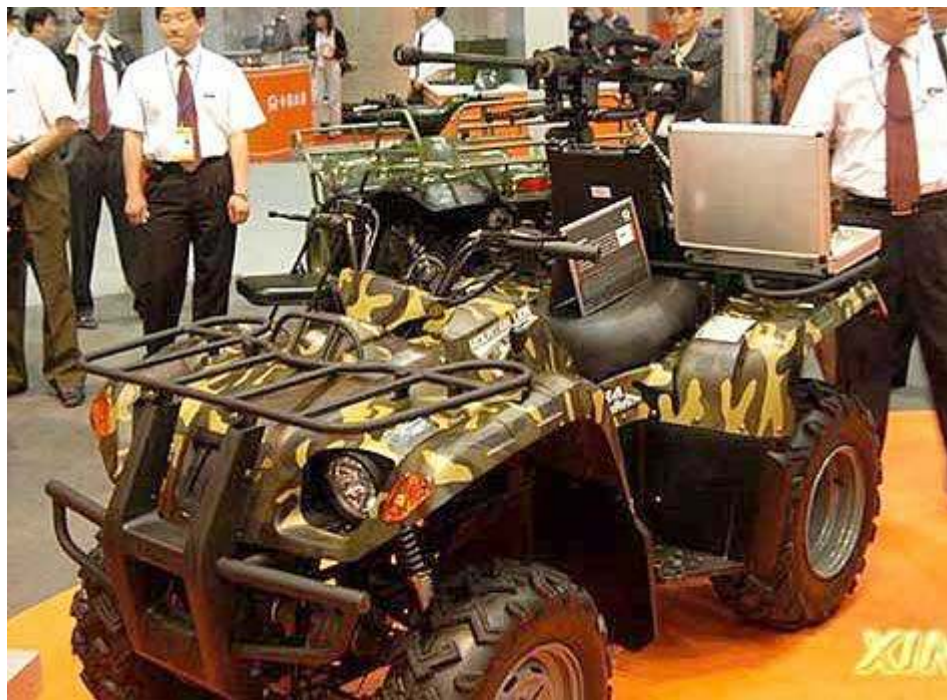
Figure 3.2 – Sino-Mab Group Industries model XZ-AT-400 4x4 ATV with a JS 12.7mm sniper anti-material rifle
